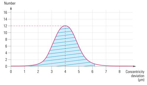
At WALTER, internal runout tests have been carried out on a HELITRONIC MINI AUTOMATION on tools with a diameter of 6 mm. The in-feed for this purpose was carried out not only via loading system but also manually (50x repetition of grinding). The runout was determined on the face of the tool.
