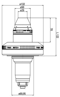
Clamping equipment\* µGrind HPS Mini for
